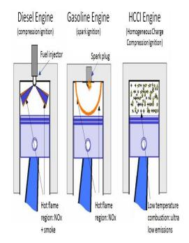
Because there is no explicit control over the combustion event in an HCCI engine, various conditions that induce combustion can be adjusted throughout the engine cycle. Gas temperature, compression ratio, residual exhaust gas, and air/fuel ratio can all be adjusted to attain desired combustion behavior. Data acquisition, processing, and actuation must happen rapidly and in real have pushed researchers to alternate LTC modes.
